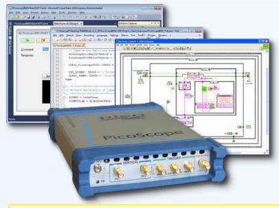
The PicoScope 9000 software can be operated as a standalone oscilloscope program and as an ActiveX control. The ActiveX control conforms to the Windows COM model and can be embedded in your own software.
