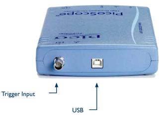
The rear panel of the PicoScope 4262 has two connections: a USB port for connection to the PC, and a BNC for an external trigger to be connected.
